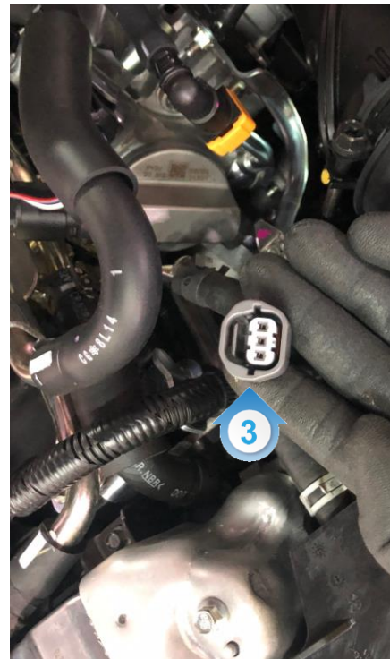
1 OP1 BOOST 2 OP2 MANIFOLD (GAUGE) 3 CAMSHAFT
