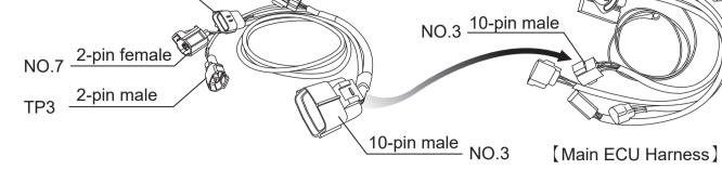
•No.3 – connect to the 10-pin female connector of the Main ECU Harness with the same labeling. •No.5 – connect to Boost sensor / Intake Temp sensor •No.6 – connect to MWI Switch control wire •No.7 – connect to Exhaust Temp sensor •TP3 – connect to Car-model Specific Wire
